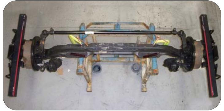
THE AMS1000 MOUNTS TO BARE AXLES IN SECONDS AND MEASURES INDIVIDUAL TOE, TOTAL TOE AND CAMBER.
