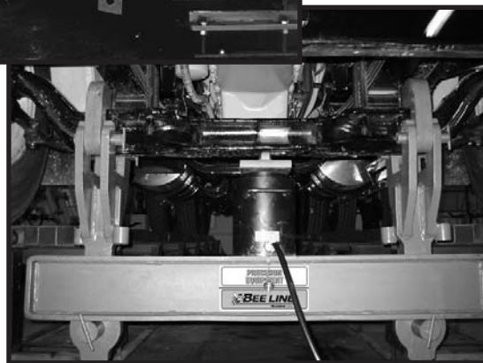
Equal camber increase with the 406 Ultra Duty Axle Tool Group.
