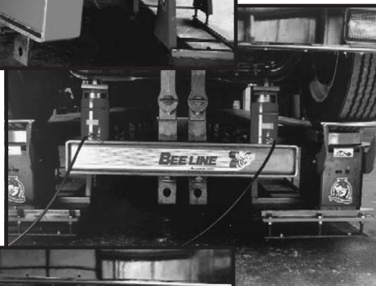
Equal camber decrease with the 405 B Axle Tool Group.
