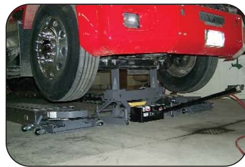
The new Bee Line 7600 Floor Jack securely lifts the vehicles front end while taking runout measurements.
