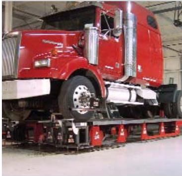
Advanced Aligners are the foundation for work in a dedicated alignment bay. With the truck elevated, you can perform computer alignments, front and rear axle camber corrections, frame corrections and rear axle alignments
