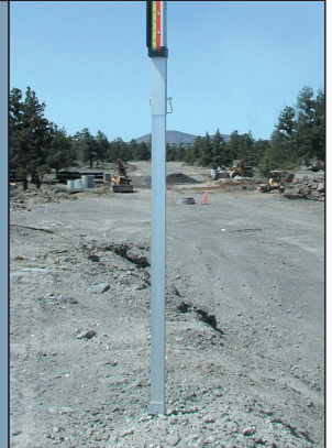
Image: shows rod extension fully extended to 4'
