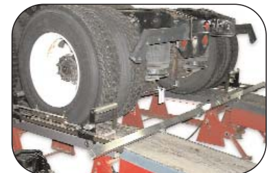
BEE LINE'S TOE GAUGE AND 21000 REAR AXLE ALIGNER CAN BE USED WITH THE ADVANCED ALIGNERS.
