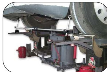
BEE LINE'S TOE GAUGE AND 21000 REAR AXLE ALIGNER CAN BE USED WITH THE ADVANCED ALIGNERS.
