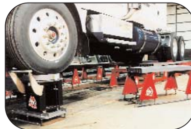
RUNWAY SECTIONS CAN BE REMOVED BEHIND THE TURNING ALIGNERS FOR EASY ACCESS WHEN MAKING CAMBER AND CASTER ADJUSTMENTS TO THE AXLE.
