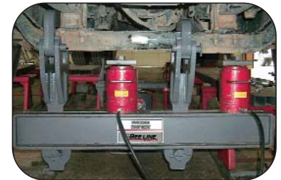
RUNWAY SECTIONS CAN BE REMOVED BEHIND THE TURNING ALIGNERS FOR EASY ACCESS WHEN MAKING CAMBER AND CASTER ADJUSTMENTS TO THE AXLE.
