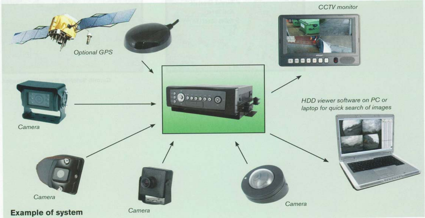
Example of camera locations connected to MDR-304
