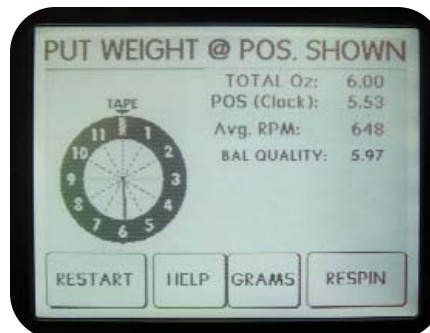
3. The touch screen indicates the position and how much weight should be placed on the wheel.
