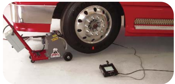
1. A spinner brings the wheel up to speed.
