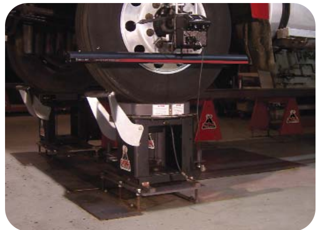
Alignment heads receive live data from the King Pin Turning Aligner.
