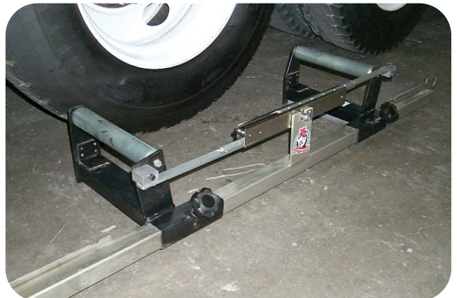
The wheel cradles feature rack and pinion frame gauges that assure accuracy when determining the axle center.
