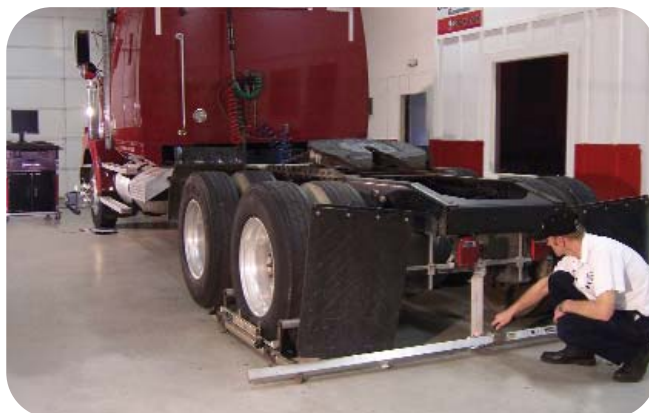
Set the rear axles with computer accuracy with the 21000 Rear Axle Aligner.
