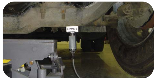
2. A sensor measures wheel vibration.
