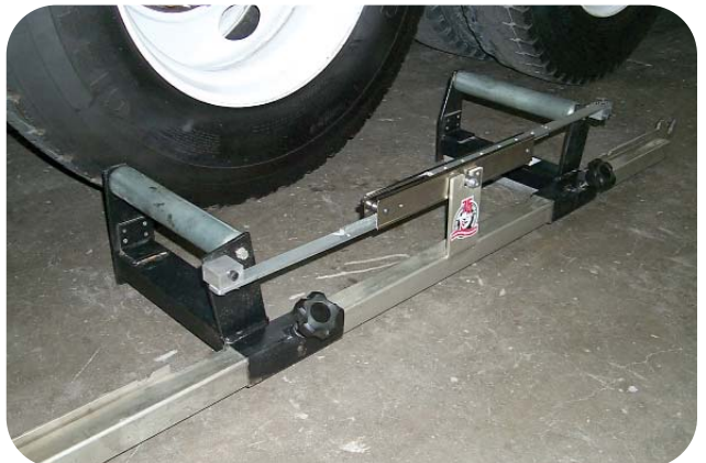
The wheel cradles feature rack and pinion frame gauges that assure accuracy when determining the axle center.
