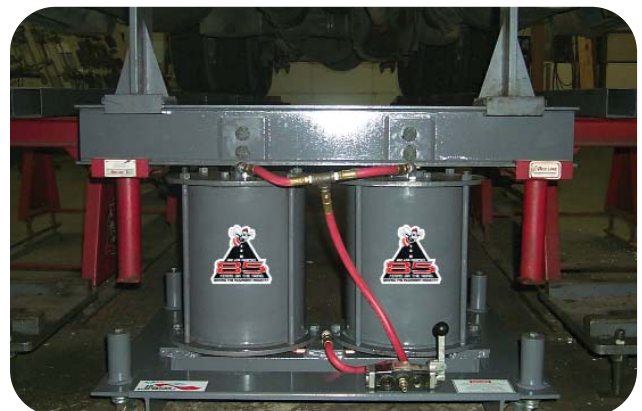
Bee Line's Heavy-Duty Air Lift Jacks provide safe and easy vehicle lifting on all Advanced Aligner Runways. The dual air lift jacks have a capacity of 3500 lbs. for each 25 lbs. of line pressure at the valve.
