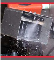
CameraWash cleans away dirt, ice, and snow from obstructing your view. Washer fluid and air pressure are mixed to keep your camera lens clean.
