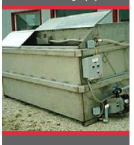
Manual and automatic brine production systems convert standard road salt into brine solution for anti-icing and de-icing applications.
