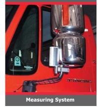
Infrared road surface temperature measuring insures accurate, real time information critical to proper deployment of anti-icing and de-icing materials.
