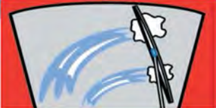
Snow build-up under wiper causes streaking.
