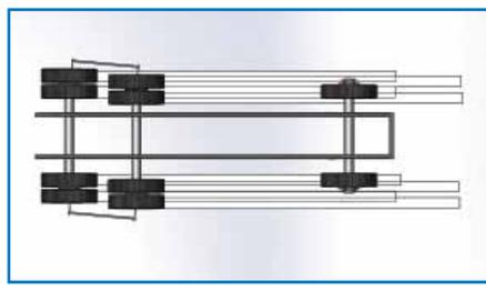
Figure D - An offset axle is automatically compensated for with Bee Line self-centering gauges. The operator aligns the laser to shoot through the rear gauge to the front target.
