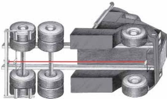
The proven 22000 lets you accurately position your rear axles perpendicular to the vehicle's centerline so the wheels travel in a straight line.
