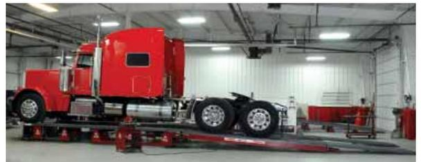
With the truck in position, Runways are hydraulically lifted with the touch of a button.
