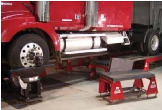
The forward runways are removable for easy access to the vehicle when making adjustments.
