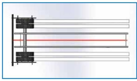
Figure C - With the Bee Line Laser Tandem Aligner, offset axles and axles with uneven spacers are set perfectly at 90° to the centerline of the vehicle. Additional axles are then simply set with a tram gauge.
