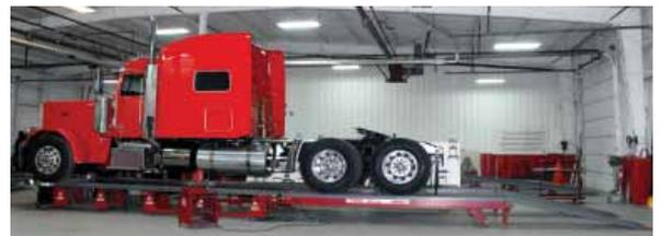
The longer design of the Space Saver lifting ramp creates a more gradual incline and requires less runway sections.
