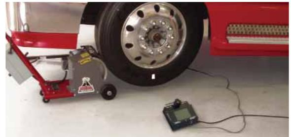
1. A spinner brings the wheel up to speed. Includes safety shield.
