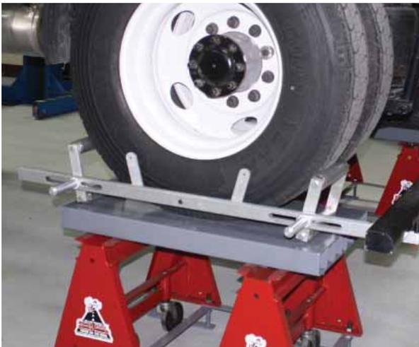
Newly redesigned cradles are just as durable, yet lighter and more easily maneuvered around the tires than ever before. The cradles feature rack and pinion gearing to assure accuracy when determining the axle center.
