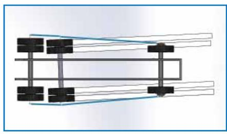
Figure A - Measuring from axle to axle will cause the operator to set both rear axles in a dog-tracking position if the first axle measured is offset or has different sized spacers.
