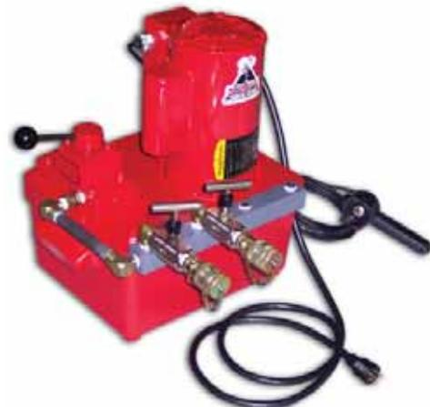
The Bee Line Electric Hydraulic Pumps are the finest pumps available on the market. The rams can operate together or separately. They operate on 115V, 10,000 PSI and require 30 amp service. The two stage system has a high volume first stage for output below 300 PSI. For efficiency, it automatically switches to a 10,000 PSI second stage. The electric pump unit is available with a solenoid control valve, or a hand held automatic release control switch valve.
