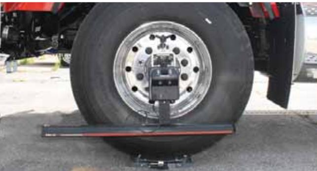
Mobile Alignments can be performed on any reasonably level surface inside or out. Our LC7500 alignment heads mount to the wheel with LC4195B.1 mounts and the wheel rests on wireless FPT8500 Turnplates.
