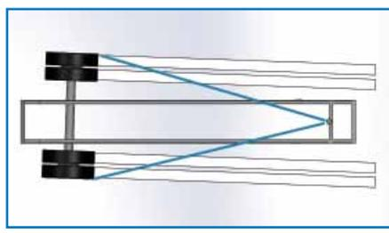
Figure B - Measuring from the king pin, or the center of the front frame, will have the same bad effects as Fig. A.
