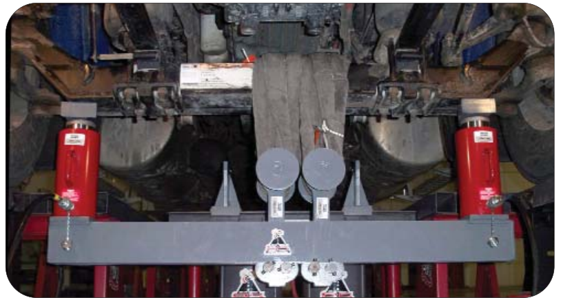
AN EQUAL CAMBER DECREASE SETUP USING THE 402 FABRICATED AXLE TOOL GROUP.
