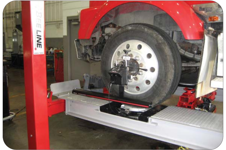
FRONT END ALIGNMENT MEASUREMENTS ARE TAKEN IN A MATTER OF MINUTES WITHOUT OBSTRUCTION.
