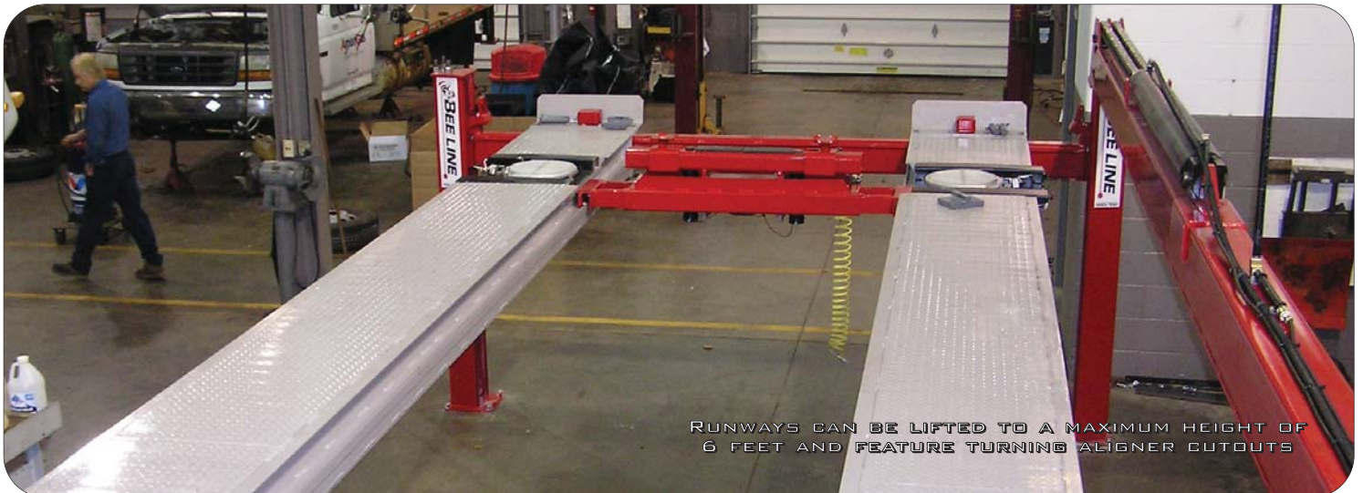
THE VEHICLE CAN BE RAISED TO A CONVENIENT WORK HEIGHT WITH EASY ACCESS UNDERNEATH.
