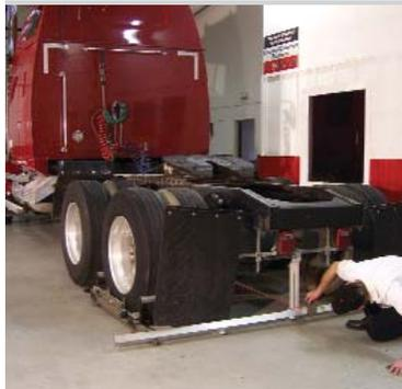
The 21000 is the fastest and easiest way to align rear axles on tractors and trailers to the centerline of the vehicle. Laser accurate readings take less than 10 minutes on the floor, runways or lift.
