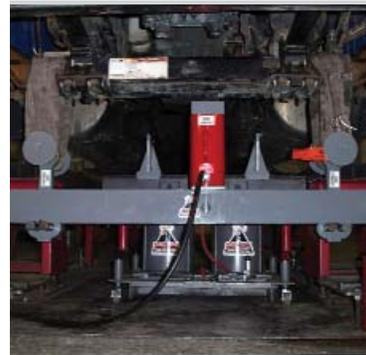
Making camber corrections on hollow fabricated axles requires our 402 Tool Group. New technology evenly distributes force without compromising the integrity of the axle.
