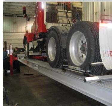
Truck lifts are available for shops that want the best of both worlds: A heavy duty four post lift for general truck maintenance and repair AND the ability to perform complete truck alignments, in the same bay, on the same machine!
