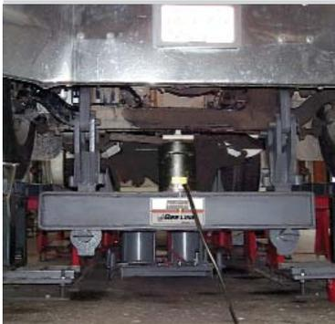
Correct Camber - the 3rd leading cause of tire wear - with our patented floating beam system. A complete alignment isn't complete without camber and caster corrections using the 406 tools.
