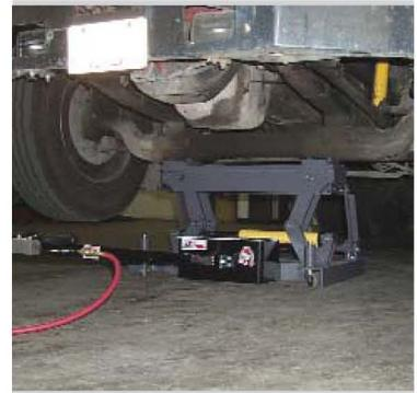
The Bee Line 7600 floor jack can lift vehicles from any two separate points of contact along its 33 inch beam. Lifting the vehicle is done with a push of a button. Slide one axle support to the center of the beam for single point lifts.
