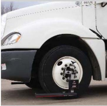
The Bee Line QTAC is the extremely fast and accurate way to diagnose potential alignment problems on heavy duty vehicles. The QTAC is extremely easy-to-use and can be taken right to the truck. "Red flag" trucks that require immediate attention.
