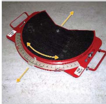
Capacity for up to 32,000 lbs per axle. Easily handles dump trucks, cement trucks, cranes and fire trucks. The rotating action is combined with lateral movement allows for the kingpin action and creates accurate, heavy duty front end alignment readings.
