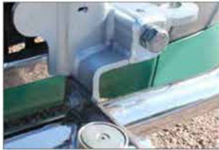
MagLatch™ secures grille guard upright with rare earth magnets
