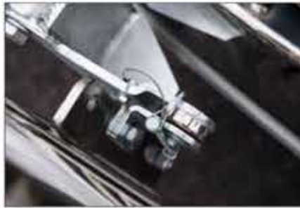
206490 safety pin adds security to the magnetic system
