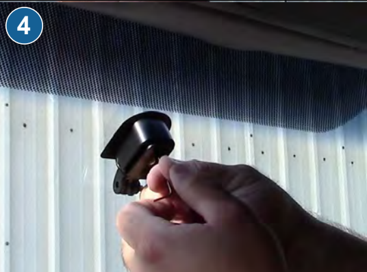
Tighten mount to the windshield lug.
