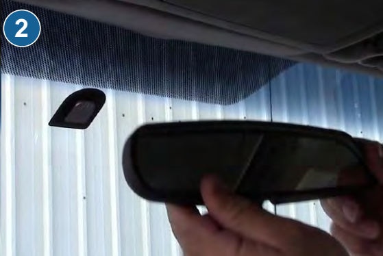
Remove the factory rearview mirror.
