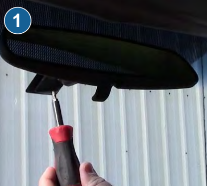
Loosen the screw on the mirror.
