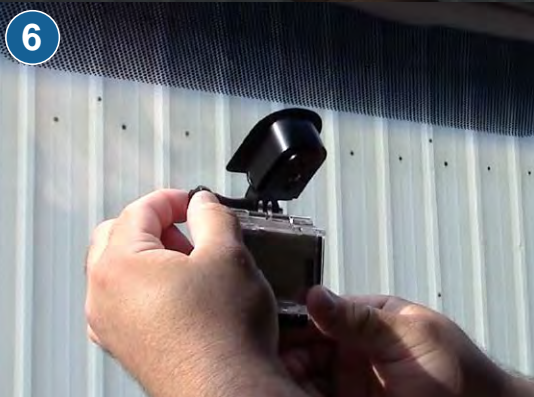
Use thumb screw to secure camera.
