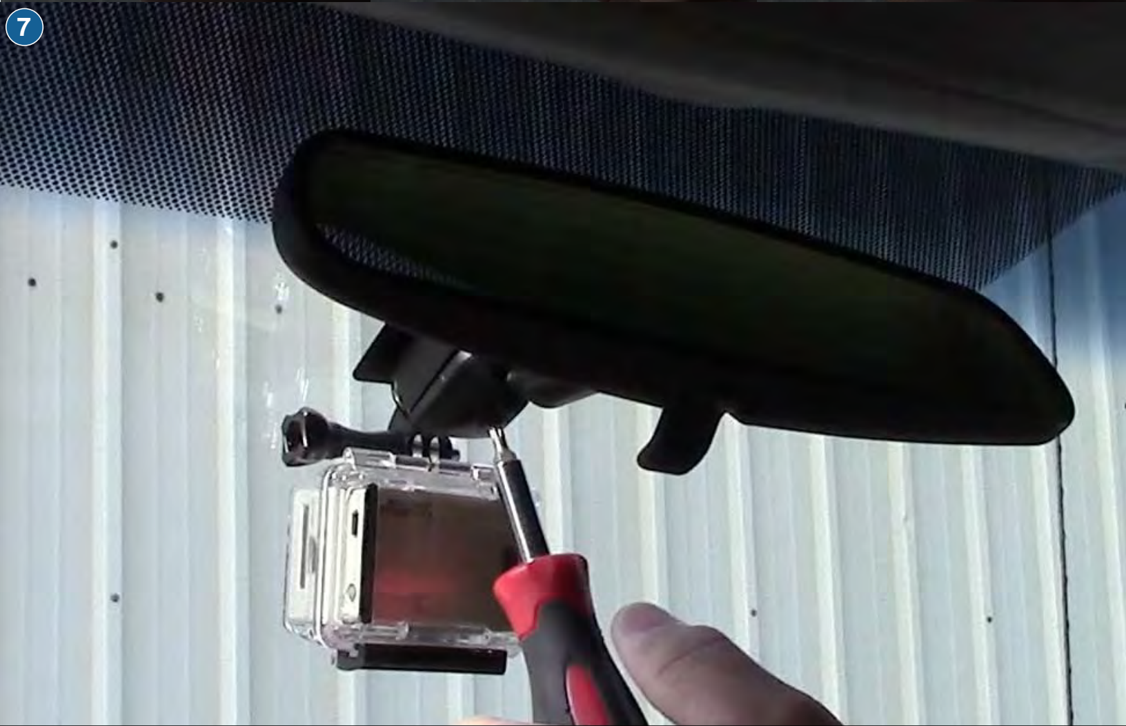
Replace the rearview mirror and tighten its attachment screw.
