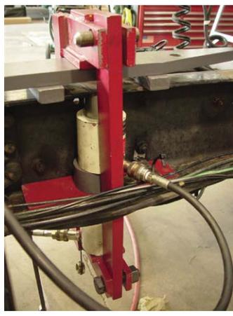
**Concentrated Pressure** – The shorter the steel bar, the harder it is to bend, as shorter lengths give less bending leverage than longer lengths. By applying 30 Tons of hydraulic pressure to a concentrated area, our flange press safely removes buckles in the flange area - the backbone of the frame.
