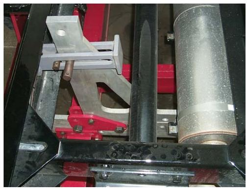
**Set Up in Tight Areas** – Extra clearance can be added to lightweight aluminum knees to make room for direct holds on the frame rail in tight areas.
