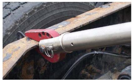
**Hand Flange** – A hand flange tool makes corrections to imperfections in flanges. An extendable handle provides leverage for the correction.
