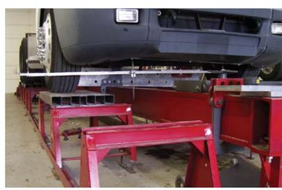
**Centerline Gauges** – Our self-centering frame gauges extend the centerline to the outside of the chassis for easy diagnosis of misalignment conditions.
