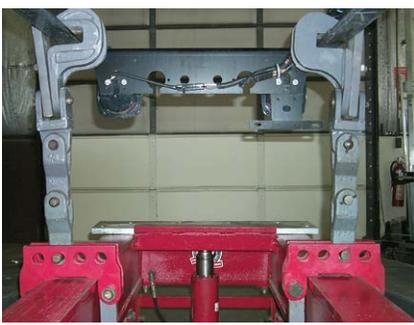
**Avoid Using Chains** – Hold downs are easily and safely made by using links and pins. Slack is removed by lowering the frame press and then applying pressure.
