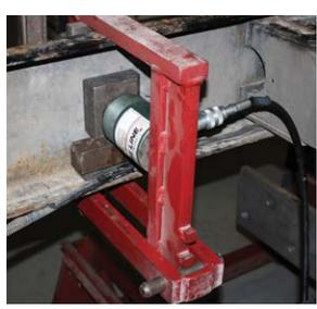
**Web Press** – Our web press provides a targeted correction to remove buckles or other damage of the web area on the frame rail using 30 ton of hydraulic pressure versus uncontrolled heat induction.
