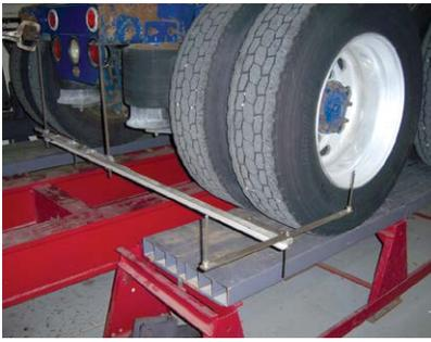
**Diagnose Diamond Condition** – A diamond sight gauge attaches to the front or rear frame gauge to diagnose a diamond condition.
