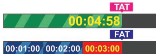
FAT storage loses nearly 1 minute of video after power shutoff.
