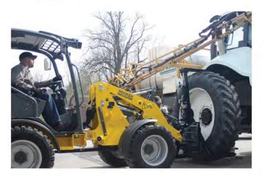
The Multi-Grip Tire Handler features a hydraulically operated gripping jaw, allowing it to easily center on the tire with a firm grip. The grabbing assembly swivels approximately 60 degrees, allowing users to easily align the wheel with the study or the wheel bolt holes on the hub. The front end loader's movement allows users to pick tires up from a flat position on the ground and rotate them to a vertical position to attach to the application unit.
