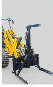
GVM's Multi-Grip Tire Handler was designed to allow users to change tires on application units, quickly, safely, and efficiently. The tire handler is able to lift and maneuver tire and wheel assemblies weighing up to 2,000 pounds, and from 56 to 80 inches in diameter. Its mounting plate allows the Multi-Grip Tire Handler to easily attach to any skid steer or front end loader with a universal mounting plate.
