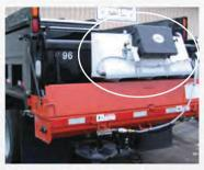
designed for quick installation and removal from the tailgate. The carrier uses four pull-pins and a lifting eye to facility ease of system installation and/or removal. Tailgate mounted system are available in 30, 70, 100, and 135 gallon sizes.
