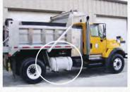
body. The pump units for these systems are mounted on the side of the dump body. Frame mounted systems are available in 35, 55 and 65 gallon sizes.
