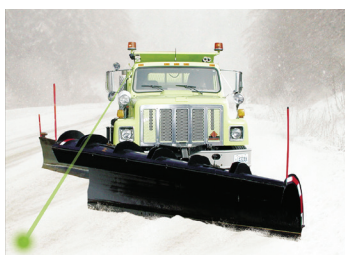
LaserLine Plow Guidance Laser
