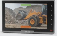
Working in conjunction with a Backeye® camera monitor system and up to two Backsense® Network radar detection systems, the on-screen display module warns the driver of obstacles in the danger zone by overlaying 5-stage audible and visual radar data onto the camera image on the monitor.
