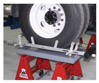
Newly redesigned cradles are just as durable, yet lighter and more easily maneuvered around the tires than ever before. The cradles feature rack and pinion gearing to assure accuracy when determining the axle center.
