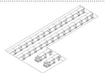
"L" Pit - Thirteen Section Drive Thru Frame Machine and Two-Section AA Pit Model with Turning Aligners for Wheel and Frame Alignment.
