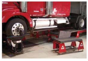
The forward runways are removable for easy access to the vehicle when making adjustments.
