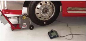
A spinner brings the wheel up to speed. Includes safety shield.
