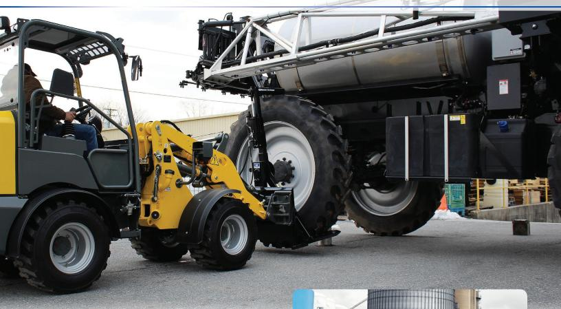
The GVM Multi-Grip Tire Handler allows users to change tires on application units quickly, safely, and efficiently. The tire handler is now available in two models and is able to lift and maneuver tire and wheel assemblies weighing up to 2000 pounds. Equipped with a universal mounting plate allowing the Multi-Grip Tire Handler to easily attach to any skid steer, front end loader, or tractor.
