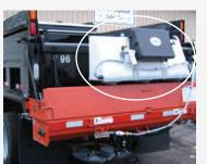
designed for quick installation and removal from the tailgate. The carrier uses four pull-pins and a lifting eye to facility ease of system installation and/or removal. Tailgate mounted system are available in 30, 70, 100, and 135 gallon sizes.
