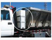
can be mounted on either the side of the dump body or between the cab and dump body. Chassis mounted systems are available in 60, 80, 90, and 120 gallon sizes.
