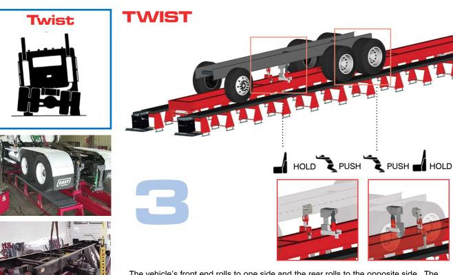
The vehicle's front end rolls to one side and the rear rolls to the opposite side. The twist is held into the chassis by the cross members. To make the correction, you must look at the strongest cross members in the chassis and where they are located since they will be the ones holding the twist into the chassis. Most vehicles will have the heaviest cross members from the cab to the back of the frame. Therefore, this is the part of the frame that you will do the correcting in.
