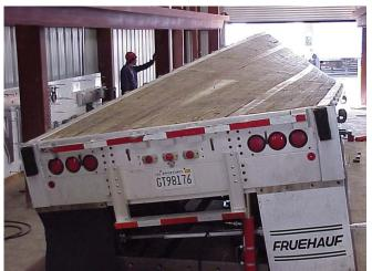
This twisted trailer is being corrected with Trailer Twisting Tools. Floor "I" Beam setup works primarily with trailer corrections.
