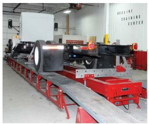
Side sway correction is made with positive locked holders and a correction crossbeam unit traveling on rollers with no friction in tooling, therefore, much less hydraulic power is needed. Bee Line equipment handles all frame damage to heavy duty trucks and trailers.
