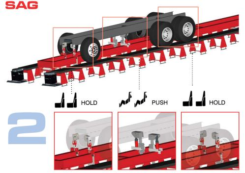
Sag is the bending of the chassis out of its true horizontal position. It can cause extensive flange damage.
