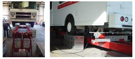
Portable Aluminum Ramps allow even the lowest profile vehicles enough clearance to traverse the Bee Line Drive Over Frame Press.
