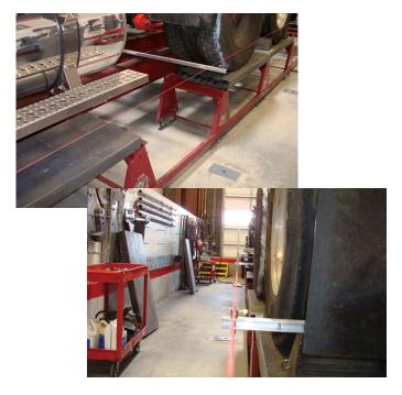
**Bee Line Tool Group #49** is designed for Heavy Duty Truck Frame Gauging. These rugged, dependable gauges quickly pin-point the damage on any truck frame and help diagnose the condition.
