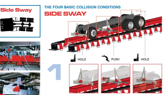
Side-sway is best described as a lateral bend in the truck chassis. This bend causes a misalignment of the centerline of the chassis, with varying degrees of flange damage, depending upon the severity of the collision.
