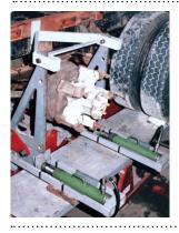
Alleviate Extra Labor - The Rear Axle Bypass setup is critical in making pushes to pinpointed areas above or around the axle without removing the axle.
