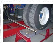
**Centerline Gauges** – Our self-centering frame gauges extend the centerline to the outside of the chassis for easy diagnosis of misalignment conditions.
