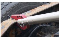
Hand Flange – A hand flange tool makes corrections to imperfections in flanges. An extendable handle provides leverage for the correction.
