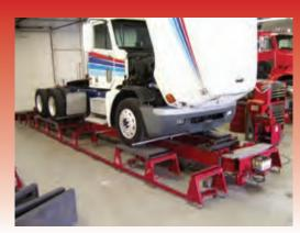
Frame gauging and equipment set up is done at a convenient height. Runways can be removed to allow easy access.
