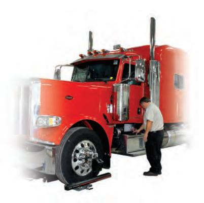
**LC7550** - Our Mobile Alignment laser guided computer alignment system features the acclaimed WindSpeed 7500 software running on a powerful Bee Line laptop computer.
