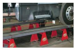
The laser beam is aimed forward in a line identical to the axle's thrust line and strikes the front target, which measures the amount of axle error from the centerline of the vehicle.
