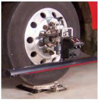
tracking and set the toe in any bay of your shop. If more extensive misalignment conditions are detected or if parts need to be replaced, the truck can be sent out to a facility with a complete Bee Line Alignment system for these corrections. Our On The Floor Alignment configuration is a fast, easy and less expensive way to make sure your trucks are performing at optimum efficiency.
