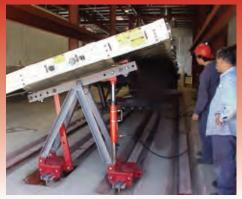
This twisted trailer is being corrected with our **Trailer Twisting** tools. Our Floor "I" Beam set up works primarily with trailer corrections. Also can be ordered for frame press.
