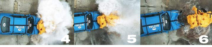
**Tested and Accepted:** EN1317-4 P4 **Impact Speed:** 110 kph Vehicle Type: 1500 kg Bullet Vehicle Impact Angle: Head-On Centre
