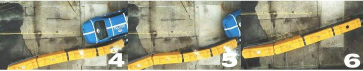
**Tested and Accepted:** EN1317-4 P4 **Impact Speed:** 110 kph Vehicle Type: 1500 kg Bullet Vehicle Impact Angle: 15° Side
