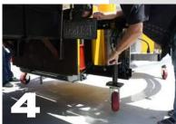
Crank jacks up and rotate for storage and insert locking pins
