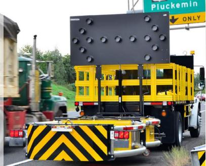
The Scorpion TMA is hydraulically powered and measures 13 feet long when fully extended, making it ideal for stationary and mobile construction zones.
