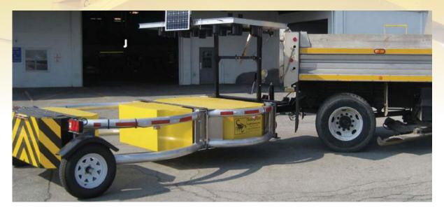
Scorpion TL-3 Trailer Attenuator with optional Arrow Board and Lift easily adapts to multiple trucks for efficient fleet management - Fast to hook up, has 45 degree turning radius, and is easy to tow and back up.
