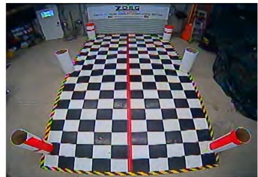
2201 102" Above Ground FMVSS 111 Compliant View Working View from 30" to 102" Licensed Under Patent 7,609,961
