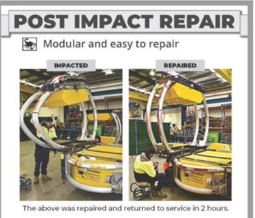
HIGHWAY ENGINEERING AUSTRALIA - AUGUST 2016 "Scorpion® TMA's not only deliver outstanding work site protection for workers and motorists alike, they have also been designed to overcome the cost and inconvenience of having to replace the entire unit even after only a minor or medium level impact... The key to their performance capabilities - both in minor and severe impacts - lies within their unique modular design."
